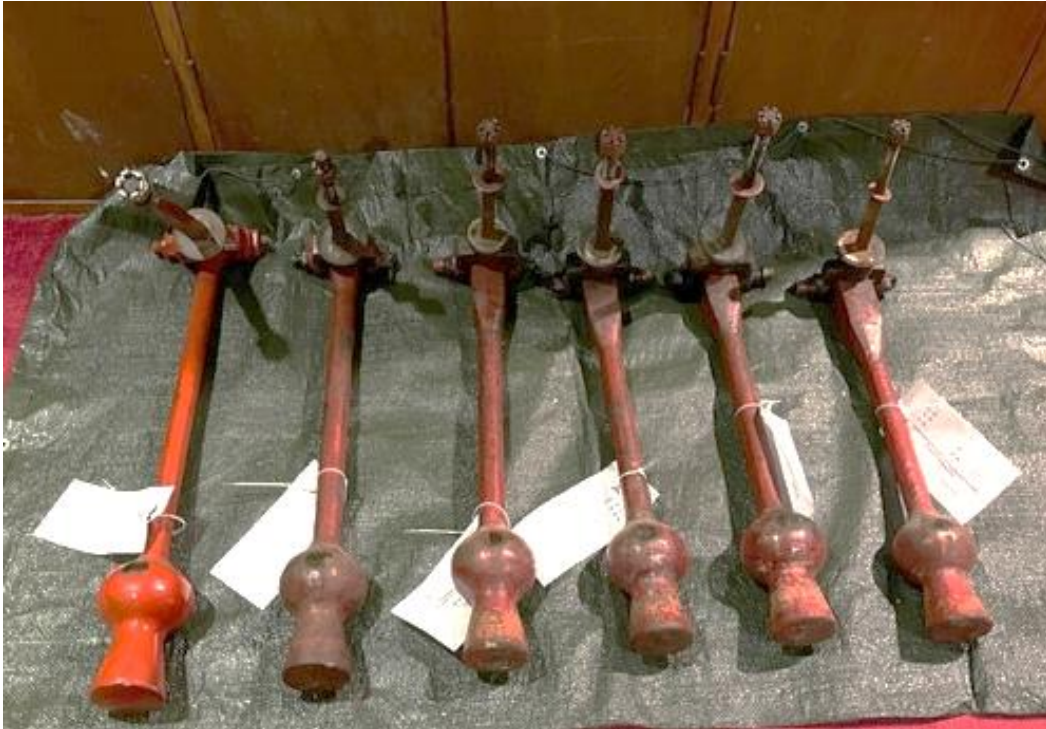
Clappers before work - you can see the worn areas on the balls. The tenor (largest bell) is a different colour as it has had some work done on it more recently than the others. They always get a coat of paint at the foundry!
